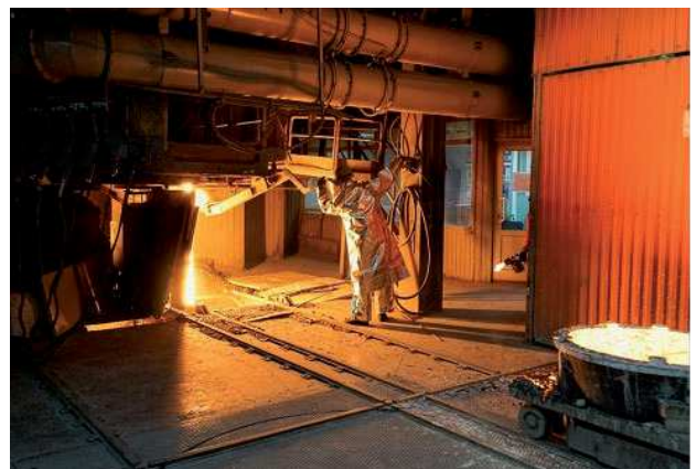
Fig. 1. The workplace of the worker during the melting of basalt rocks
