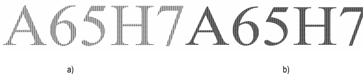
Figure 6. Grating of the same color as background being placed over the text. Images on (a) and (b) have different width of grating lines
