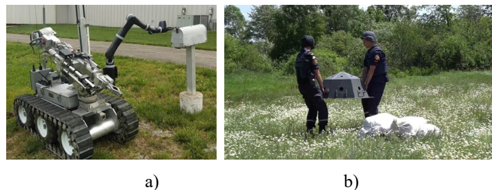
Figure 1. Examples of bomb disposal devices: a) a prototype of a smart cone device from the National University of Civil Defence of Ukraine, Ukraine (courtesy of Yevhen Stetsiuk), and b) remotely controlled bomb disposal robot Andros Wolverine 6X6 (source [27]).
