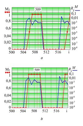
Fig. 3. The dynamics of discrete values of the combined risk of instantaneous action (2) and the CRLR window measure (4) for two values of the *w* parameter: a - w = 1; b - w = 0
