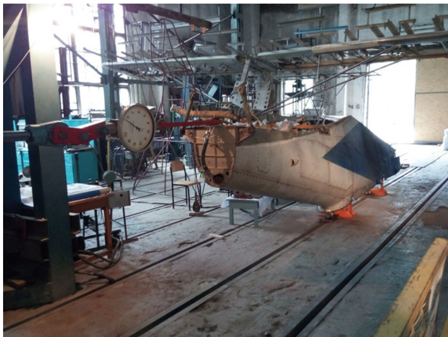
Fig. 2 General view of the test bench for measuring aircraft engine thrust
