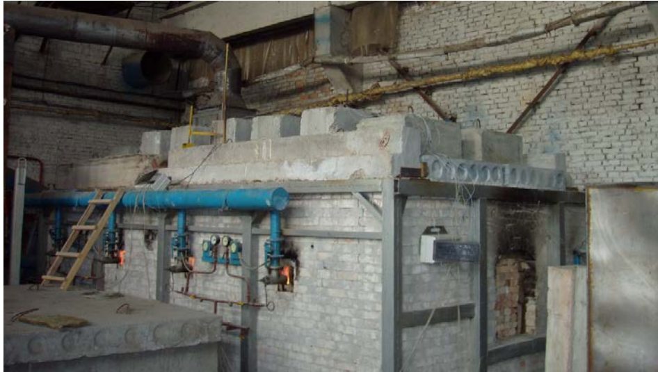
Fig. 2. Appearance of samples on the furnace under load
