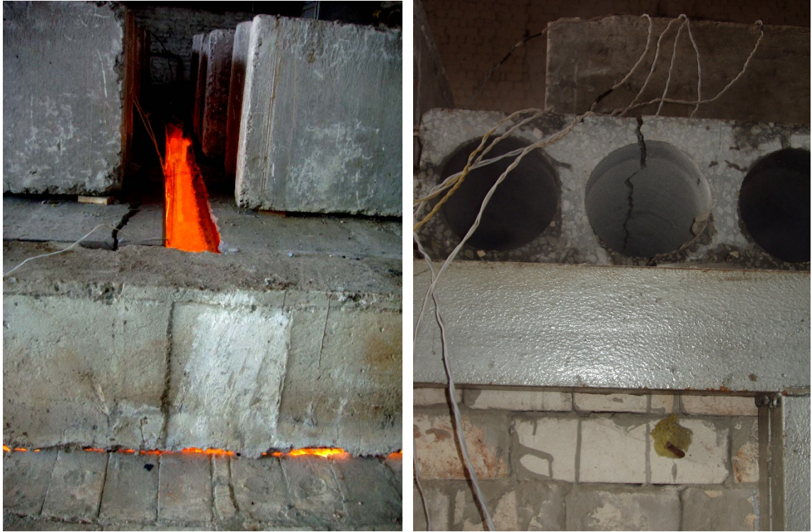
Fig. 4. Area of collapse of sample number 2
