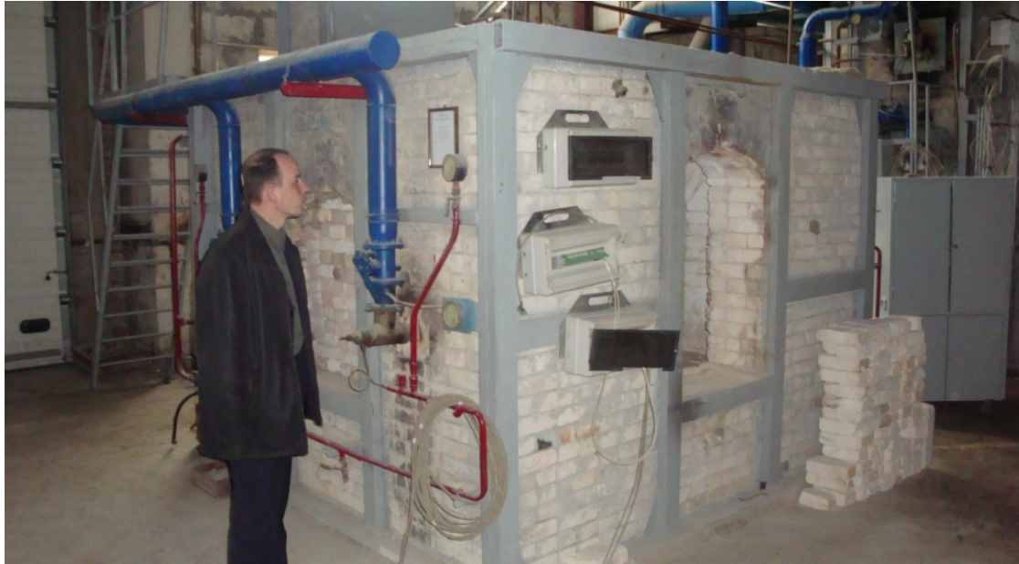
Fig. 1. A fire furnace for fire resistance of reinforced concrete structures research
