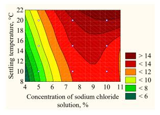
Fig. 5. Dependence of wax yield on the concentration of sodium chloride solution and settling temperature
