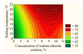
Fig. 6. Dependence of wax melting point on the concentration of sodium chloride solution and settling temperature
