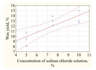
Fig. 1. Dependence of experimental data on the wax yield on the concentration of sodium chloride (experimental data and approximating curves)
