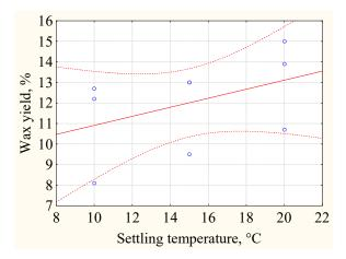
Fig. 3. Dependence of experimental data on the wax yield on settling temperature (experimental data and approximating curves)
