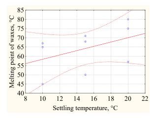
Fig. 4. Dependence of experimental data on the melting point of waxes on settling temperature (experimental data and approximating curves)
