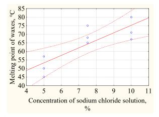
Fig. 2. Dependence of experimental data on the melting point of waxes on the concentration of sodium chloride (experimental data and approximating curves)
