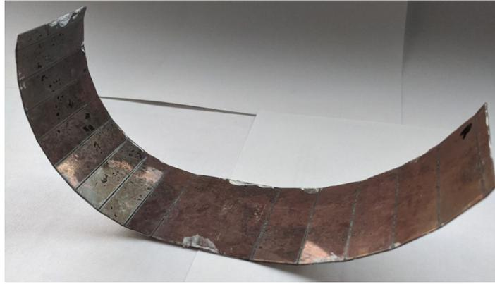
**Fig. 5.** Sample shape at irradiation with 15 mm pitch (right side) and 10 mm pitch (left side)
