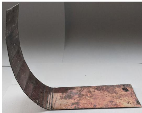
**Fig. 6.** Sample shape at irradiation with variable pitch of 20, 15, 10, 5 mm (in pairs starting from edge to middle)**Table 5.** Results of formation with variable pitch of 20, 15, 10, 5 mm (in pairs starting from edge to middle)
