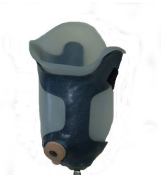
Fig. 2. Frame outer sleeve of the hip prosthesis with a silicone contact sleeve
