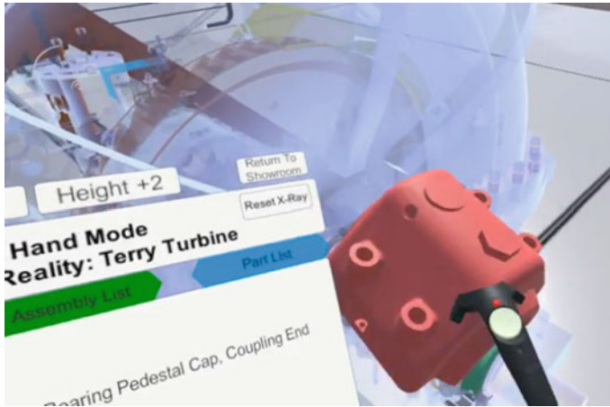
Fig. 5 EPRI virtual reality training for terry turbine maintenance (Example 3)
