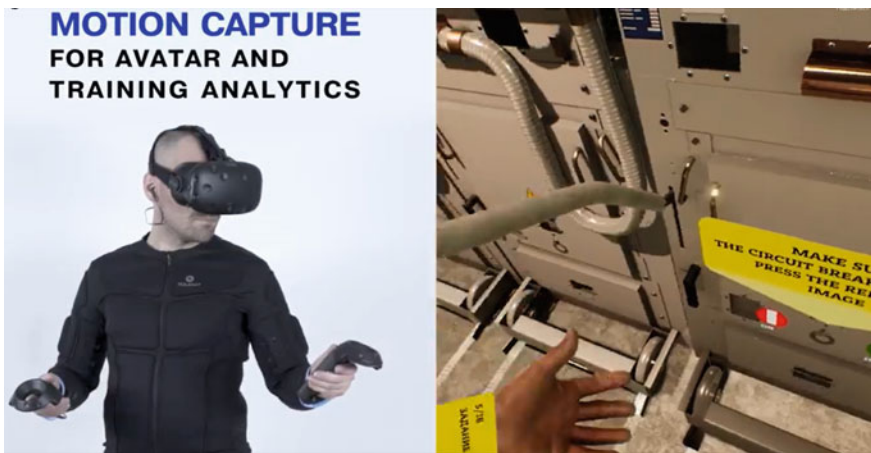
Fig. 1 The Teslasuit smart suit for a thermal power plant [51]
