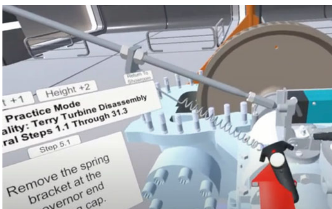
Fig. 4 EPRI virtual reality training for terry turbine maintenance (Example 2)
