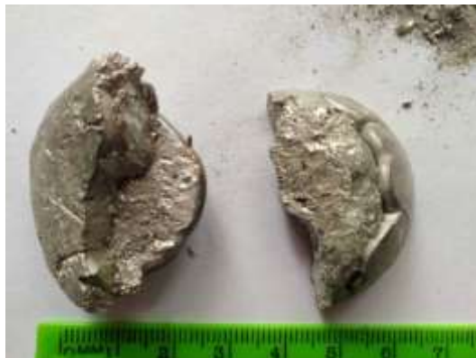
Figure 3. Alloy of hydrogen hydride carrier, which is smelted in the form of ingots
