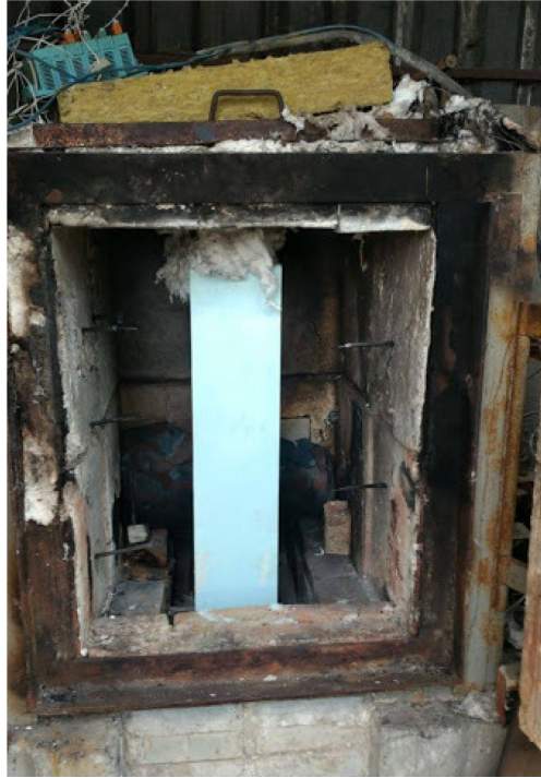
Fig. 3. Ready to test I-beam placed in the furnace
