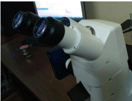
**Fig. 4.** Metallographic microscope ZEISS AXIO Vert.A1
