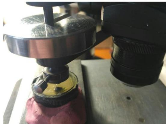
**Fig. 5.** Measurement of microhardness on samples
