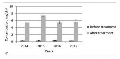
Fig. 1c. Average annual concentration dynamics of nitrate nitrogen (c) in wastewater before and after treatment (Iurchenko et al., 2020)
