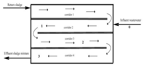
Fig. 2. Scheme of the flows in aeration tank at the Kharkiv WWTP and sampling points during research (sampling points 0 – etntering sewage, 1 – 2-nd corridor, 2 – 3-rd corridor, 3 – the end of 4th corridor)
