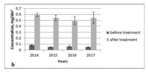
Fig. 1b. Average annual concentration dynamics of nitrite nitrogen (b) in wastewater before and after treatment (Iurchenko et al., 2020)
