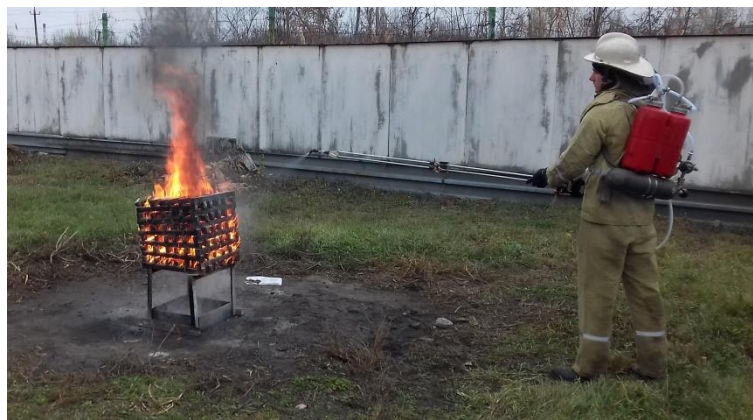
Fig. 1. Extinguishing the simulation fire 1A by the installation with the extended barrel of the cranked type for extinguishing by gel-forming compositions
