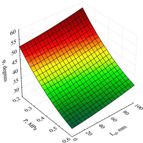
Fig. 2. Dependence of the twisting angle  $\varphi$  on the pressure in the sleeve and the length of the defect on the base
