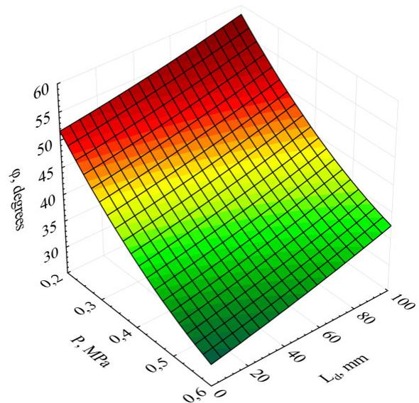
Fig. 3. Dependence of the twisting angle  $\varphi$  on the pressure in the sleeve P and the length of the defect  $L_d$  on the weft
