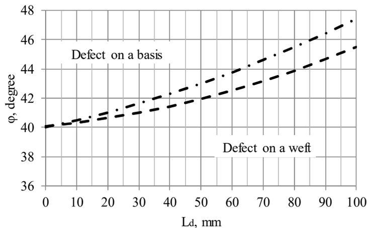
Fig. 4. Experimental dependence of the angle of twist of the sleeve on the length of the defect on the base and on the weft
