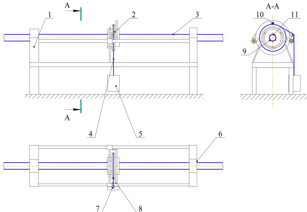
Fig. 1. Scheme of the experimental installation to determine the flexible pipeline twisting angle: 1 – installation frame; 2 – active housing; 3 – sample of the flexible pipeline; 4 – cable; 5 – cargo; 6 – cylindrical clamps; 7 – rolling support; 8 – cable guide; 9 – fixators; 10 – deformation meter; 11 – clamp
