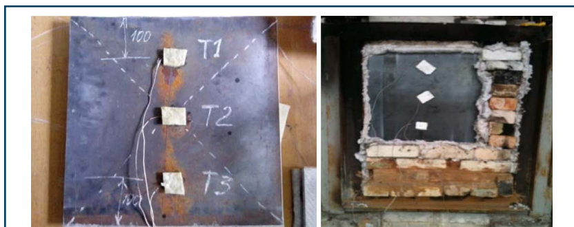
○ Fig. 4.6 Layout of thermocouples from the unheated surface of the steel plate before the test
