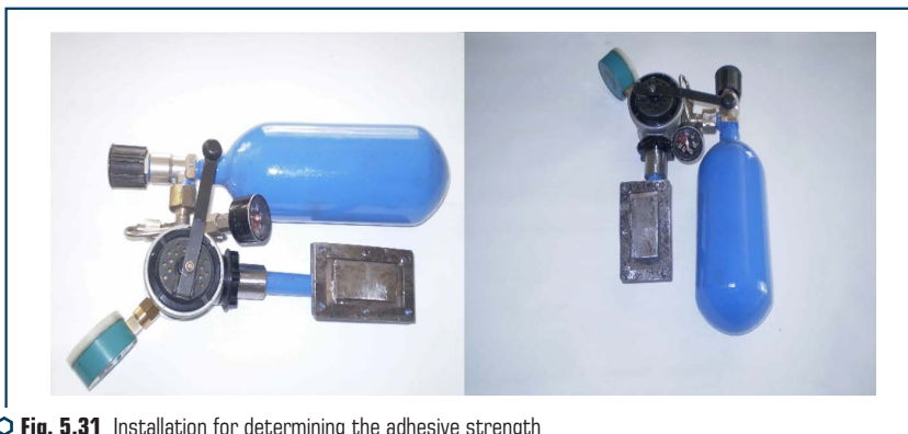
○ Fig. 5.31 Installation for determining the adhesive strength of coatings of fire-retardant steel structures
