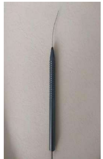
Fig. Working electrode for ophthalmic monopolar electrocoagulation with high-frequency current
