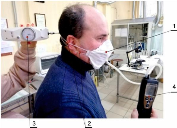
**Figure 3.** General view of laboratory tests. Note: 1 = respirator model Standard 213 FFP2 NR (LLC SPE Standart, Ukraine); 2 = elastomeric head straps; 3 = dynamometer DU-100 (PromTechniMashPrylad, Ukraine); 4 = differential pressure gauge Testo 512 (TESTO AG, Germany). The full colour version of this figure is available online.
