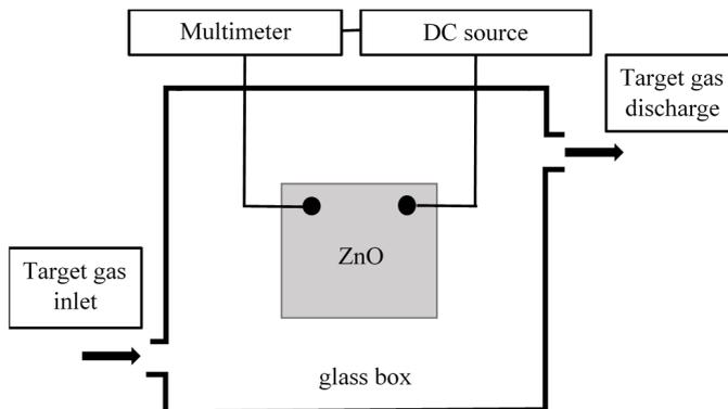
Fig. 2. Block diagram of the installation for studying the sensitivity of the gas sensor
