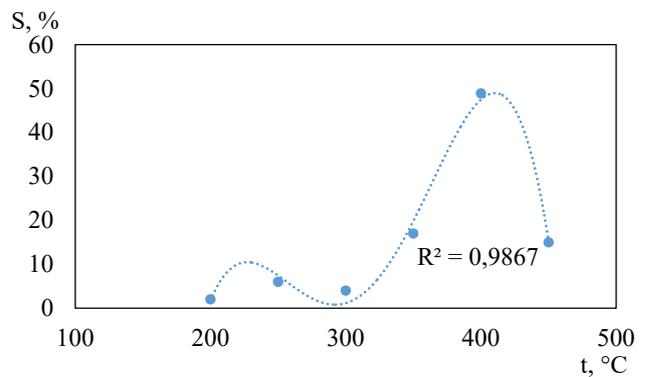
Fig. 4. ZnO-based gas sensor sensitivity
