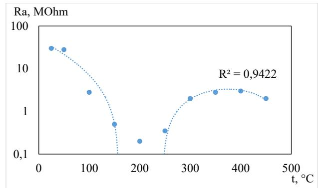
Fig. 3. Dependence of ZnO-based gas sensor resistance on substrate temperature
