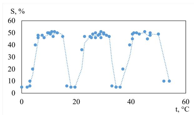
Fig. 5. Response of the sensitivity of the ZnO-based gas sensor to the target gas under repeated exposure (500 ppm gas concentration)
