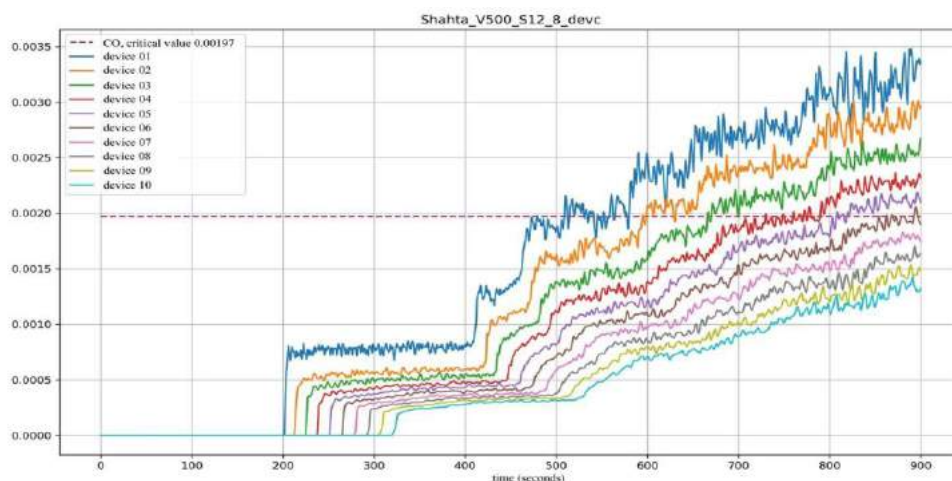
Figure 2: Dynamics of CO at the site 0 to 95 m from the source of the fire in the working with an area of 12.8 m 2 and airflow of 500 m 3 /min as evidenced by the sensors located at the top of the vault. The dashed line indicates the CO level that exceeds the MPC at the workplace
