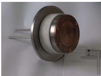
Fig. 2. Material-saving magnetron for vacuum unit VUP-5M
