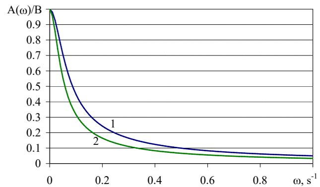
Fig. 2. Relative amplitude and frequency characteristics of a fire: 1 –  $\tau=20$  s; 2 –  $\tau=30$  s
