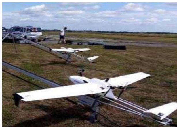
Figure 1.1 shows an aircraft-type UAV of the Cetus model of the Abris company (Ukraine)
