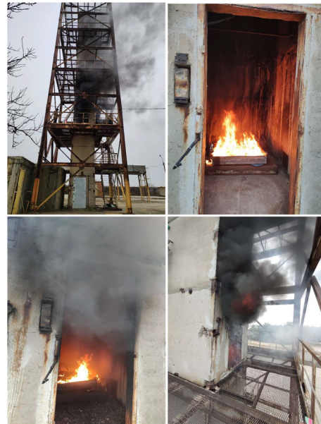
Fig. 5. Photo of the cable tunnel during the experiment
