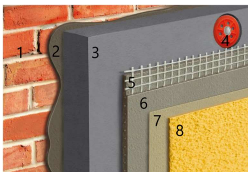
Fig. 1 Facade insulation system components. (1) The foundation of masonry; (2) Mineral glue „Sakret BK“, yield about 5 kg/m 2 ; (3) Gray polystyrene foam „EPS 70“ thickness 180 mm, density 14.0 kg/m 3 ; (4) Plastic studs, yield 4 pcs/m 2 ; (5) Sakret fiberglass mesh, area weight about 160 g m 2 . Manufacturer UAB Sakret LT; (6) Mineral reinforcement plaster „Sakret BAK“, yield about 5 kg/m 2 ; (7) Polymeric primer before decorative plaster Sakret PG yield about 0.25 l/m 2 ; (8) Decorative plaster Sakret SBP, yield about 4 kg/m 2 .
