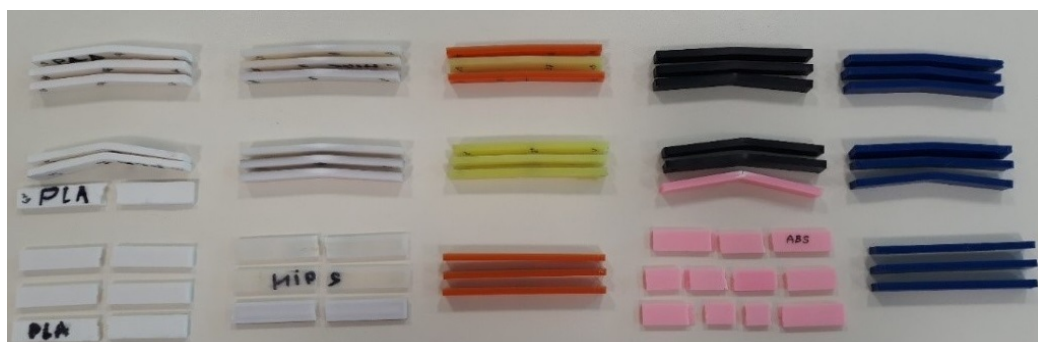
Fig. 1. Samples after bending tests. Top-down: at + 22 °C, 0 °C, -40 °C. From left to right: PLA, HIPS, SBS, ABS, PETG
