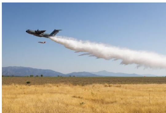
Pic.1 Testing A400M roll-off kit
