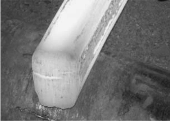
Fig. 1. Cracking at the front end of breakdown after three passages: 60C2 steel, 130×130 mm billets
