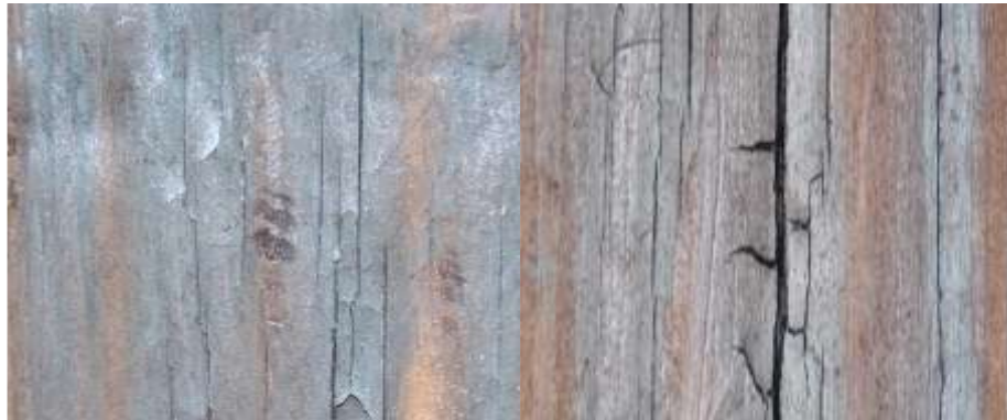
Fig. 1. Views of pine wood specimen after affected with the heat fluxes of 8 kW/m 2
