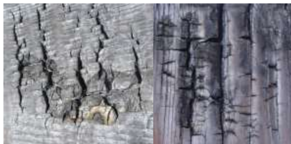
Fig. 2. Views of pine wood specimen affected with the heat fluxes of 10 kW/m 2
