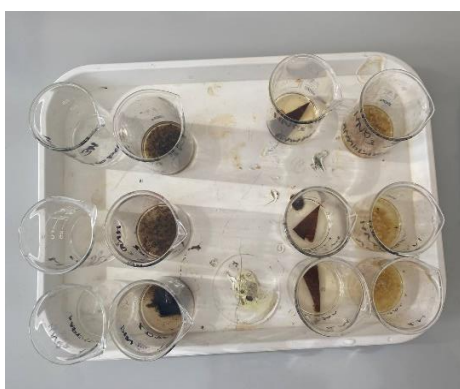
Picture 2 Samples in 1M, 2M, 3M solutions of \text{HNO}_3
