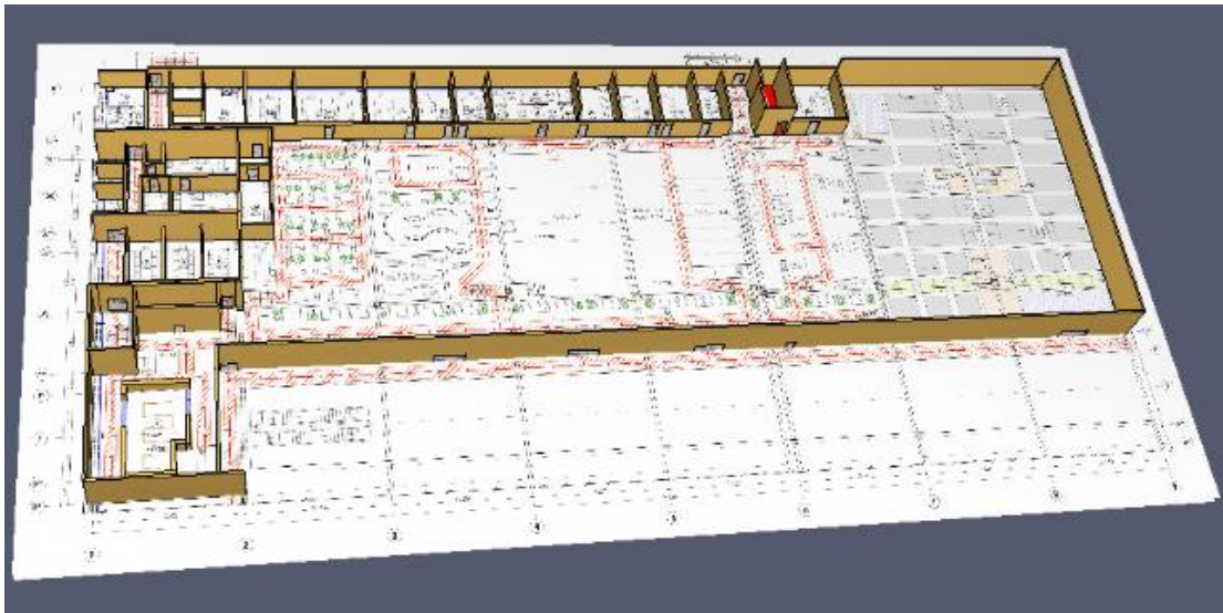
Figure 1 – Room model for simulation of the dynamics of fire hazards
