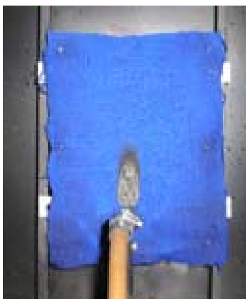
Fig. 2. Appearance of the samples PROBAN after testing
