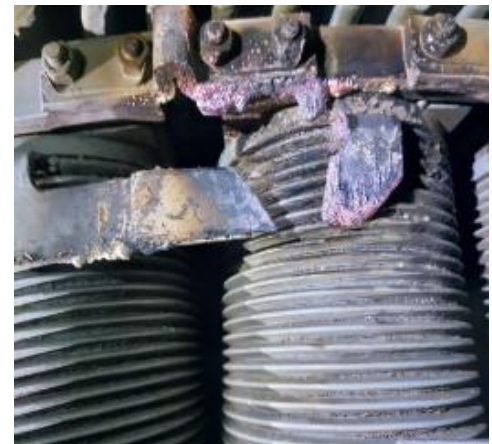
Fig. 1. Cliff of the jumpers of the rotor damper winding
