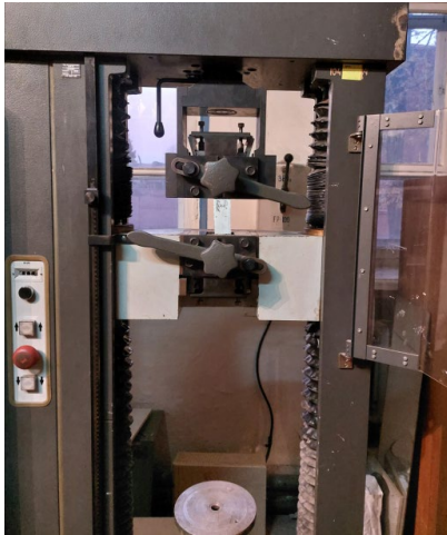
Fig. 1. Fixation of prototypes in a burst test machine
