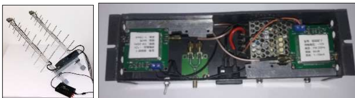
Figure 3 – Appearance, antenna system, and element base of the decimeter and meter wave range amplifier
