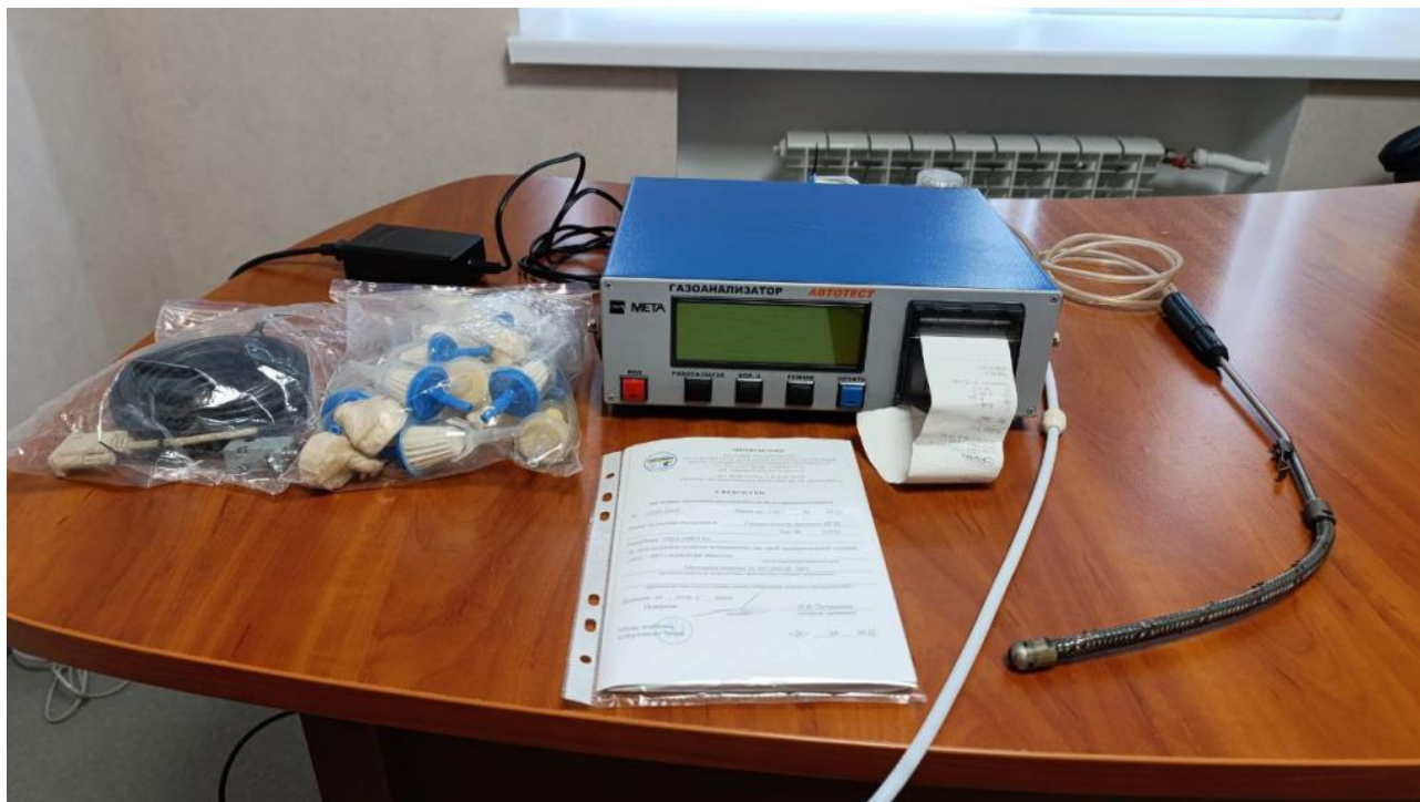
Figure 5 – The 4-component gas analyzer Autotest 02.02 for the mobile test bench
