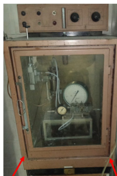
Gas-air mixture unit Test chamber
