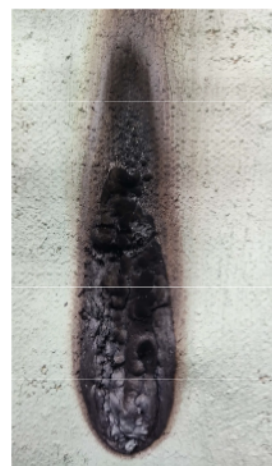
Fig. 8. Test results for determining a biocomposite based on tarpaulin fabric: a – test structure, b – burner effect on the material, c – coke foam layer after combustion
