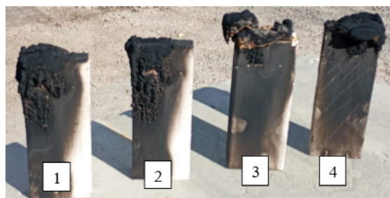
Fig. 5. Samples of wood biocomposites after thermal treatment: 1 – MDF, 2 – particleboard, 3 – wood, 4 – plywood
