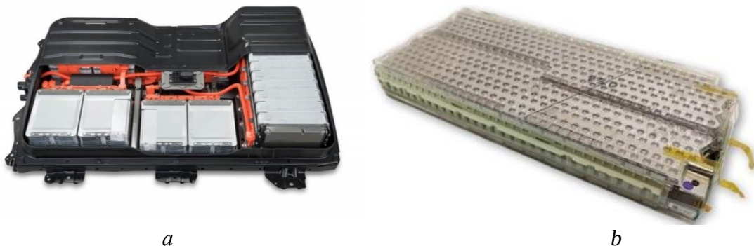
Figure 1 – Contents of the battery pack: a – Nissan Leaf; b – Tesla car module
