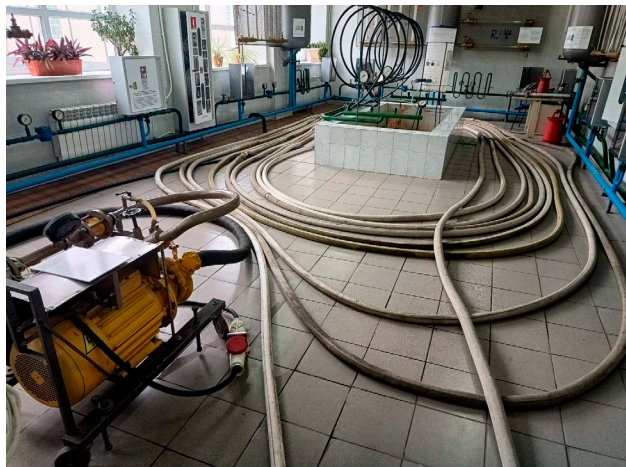
Fig. 2. Laying a hose line of pressure fire hoses with a diameter of 51 mm
