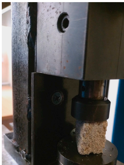
Fig. 7. Determining the compressive strength of biocomposites
