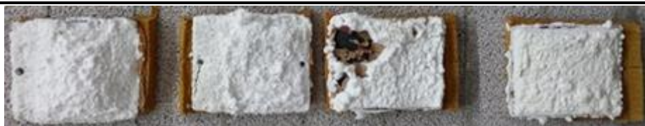
Fig. 2. Control samples after fire resistance tests.
