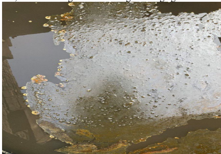
Fig. 4. Protective gel film formed on the surface when extinguishing a model fire 55B1 with a solution based on a gel concentrate of polyacrylamide and a general-purpose foaming agent.
