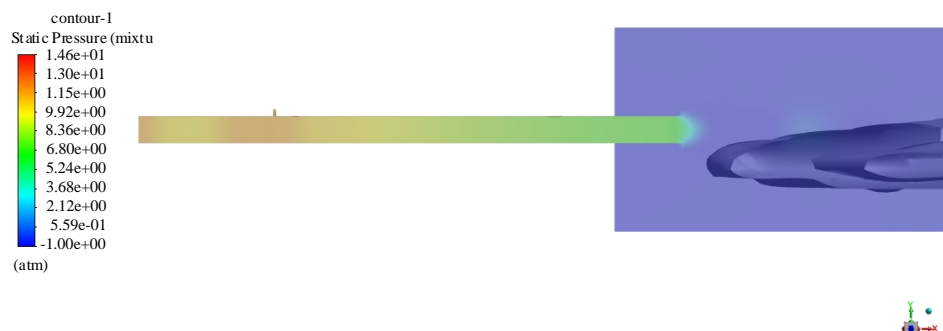
Fig. 9. Distribution of the liquid during the generation of fine water mist from the nozzle of the fire-extinguishing system under the action of shock waves at the simulation time of 5.24 ms
