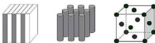
Figure 4. Schematic diagram of one-dimensional, two-dimensional and three-dimensional phononic crystals
