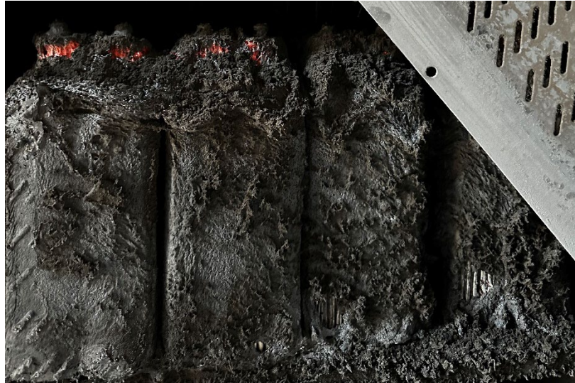
Fig. 14. Condition of the 12V 100 A#2 batteries of the PSS SHZh power supply cabinet upon completion of experiment No. 9.
