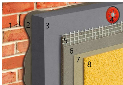
Fig. 1 Facade insulation system components. (1) The foundation of masonry; (2) Mineral glue „Sakret BK“, yield about 5 \text{ kg/m}^2 ; (3) Gray polystyrene foam „EPS 70“ thickness 180 mm, density 14.0 \text{ kg/m}^3 ; (4) Plastic studs, yield 4 pcs/ \text{m}^2 ; (5) Sakret fiberglass mesh, area weight about 160 \text{ g/m}^2 . Manufacturer UAB Sakret LT; (6) Mineral reinforcement plaster „Sakret BAK“, yield about 5 \text{ kg/m}^2 ; (7) Polymeric primer before decorative plaster Sakret PG yield about 0.25 \text{ l/m}^2 ; (8) Decorative plaster Sakret SBP, yield about 4 \text{ kg/m}^2 .
