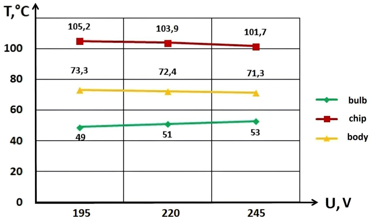
Fig. 7. Dependence of the temperature of the LED lamp elements on the supplied electric voltage.
