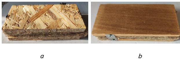
Fig. 2. General view of SIP panel samples: 1 – based on OSB board and hemp insulation; 2 – based on plywood and hemp insulation
